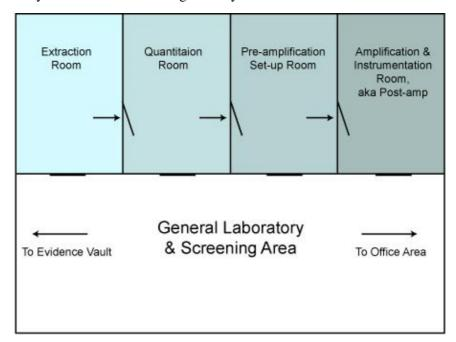
A very generic schematic of a laboratory layout that would comply with standards to prevent contamination. Note the one-way flow of the samples. Additional rooms may be present for reagent preparation, film development, computer use, etc. Each area should have dedicated equipment, reagents, and PPE.
